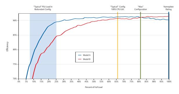
Figure 9. Power supply efficiency can vary significantly depending on load and power supplies are often sized for a load that exceeds the maximum server configuration.
