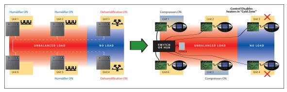
Figure 15. System-level control reduces conflict between room air conditioning units operating in different zones in the data center.
