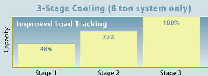
*A unique compressor staging system utilizes independent 3-ton and 5-ton circuits to provide better control of room conditions. The unit microprocessor continuously monitors recent cooling operation, and selects the most economical cooling stage to satisfy demand.*
