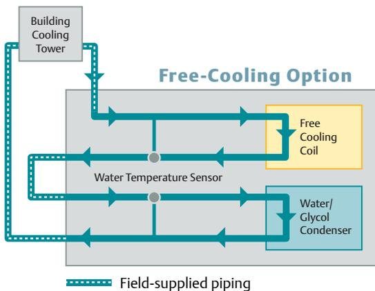
When water temperature goes below 45°F, cooling switches over to Free-Cooling operation. A separate chilled water source can also be used with Air-Cooled system. Note: Special cupro-nickel free-cooling coil must be specified when applied to open cooling tower.
