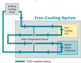
When water temperature goes below 45°F, cooling switches over to Free-Cooling operation. A separate chilled water source can also be used with Air-Cooled system. Note: Special cupro-nickel free-cooling coil must be specified when applied to open cooling tower. You will find a full-range of monitoring and control systems, communications modules designed to interface Liebert equipment with a variety of building management systems, plus stand-alone monitoring, control and leak detection devices.
