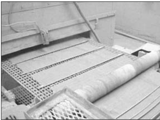
Figure 3. Batteries are created by rolling paste onto a gride of positive and negative plates that then converts chemical energy directly to electrical energy.
