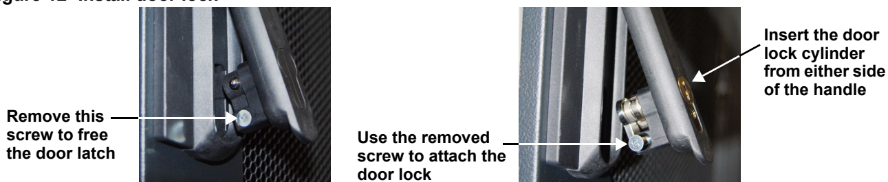
Figure 12 Install door lock
