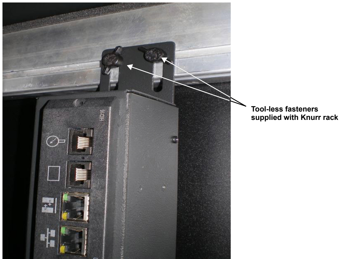
Figure 4 Attaching a Liebert MPH to a Knurr Miracel horizontal frame member
