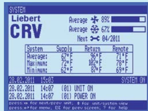
A single view shows the average, minimum, and maximum temperature of every 2T rack sensor in a single- or multi-unit system.
