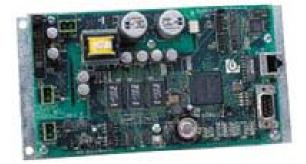
**DESCRIPTION** The OpenComms Network Interface Card provides Network and Modbus connectivity for your Emerson Network Power equipment. Operating status is monitored and alarms are communicated via the network, using SNMP and/or HTTP protocols and over RS-485 using Modbus protocol.
