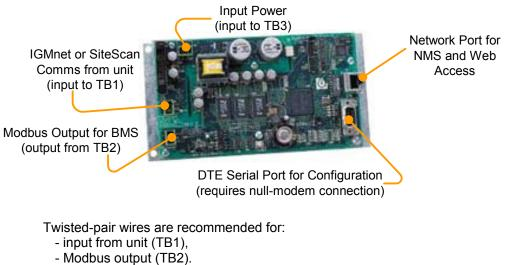
Note polarity as indicated. Maximum cable run: 1000ft (328m) @ 22AWG.
