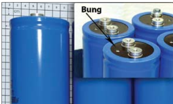
Figure 3A. Rubber bung is shown for the DC electrolytic capacitor.
