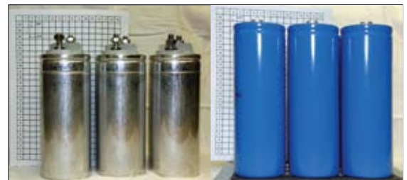
Figure 2. The shiny metal case is the AC polymeric film capacitor and the blue insulated metal case is the DC electrolytic capacitor. The grid in the background is 1 cm by 1 cm squares.
